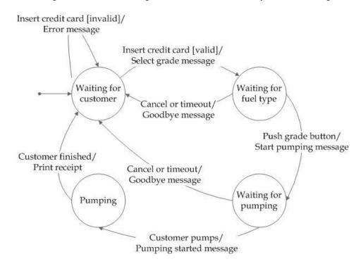
Assume that you want to develop the minimum number of tests to cover each transition in the state transition diagram. Assume further that each test must start at the beginning state, waiting for customer, and each test ends when a transition arrives at the beginning state. How many tests do you need?
