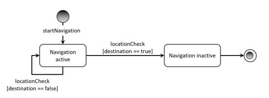
Now, a new requirement turned up. It shall be possible to interrupt the navigation in order to change the destination or to abort the navigation. The test team decided to add a new transition triggered by the event "userInterrupt", plus a new state "Navigation interrupted" to the existing MBT model. Therefore, the test team created a second version of the MBT model:
